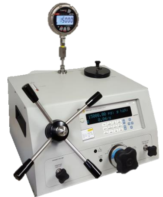
Wide Rangeability Assures Wide Workload Coverage - Calibrations Up To 15,000 PSI
